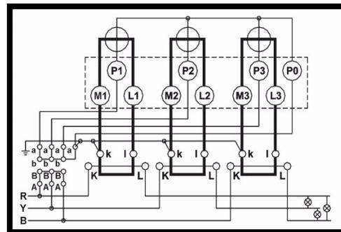
FIG. iii 3PHASE 4WIRE WITH CT & PT
