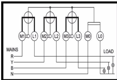
FIG. v 3PHASE 4WIRE - WHOLE CURRENT
